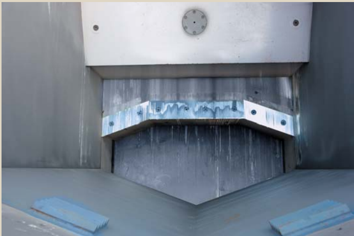
View of the cutting blades, which are the full width of the loading chamber
