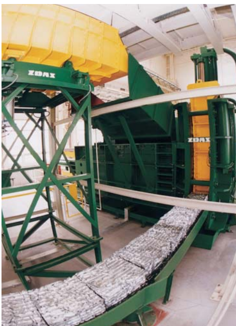
ZDAS CPS 320 baling press in a pressing shop of a large automotive manufacturer
