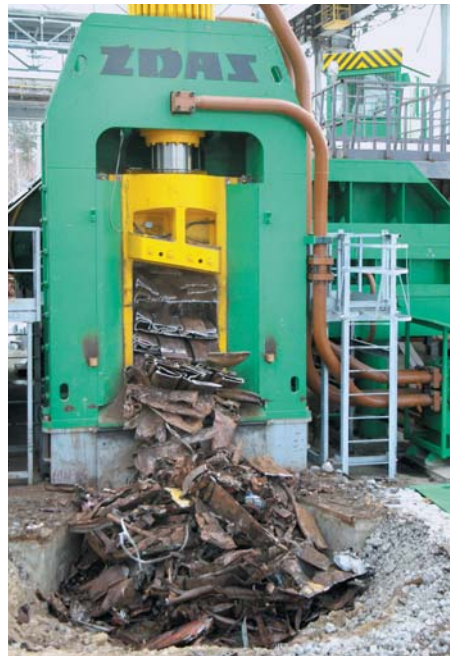
Pushing out the cut scrap
