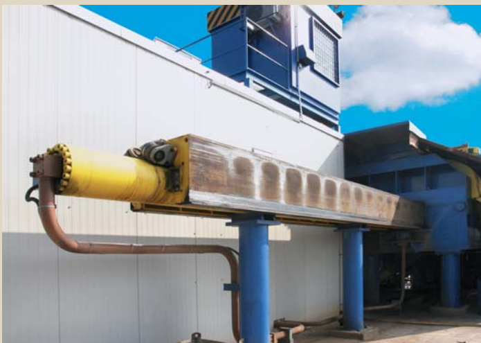
The pusher's hydraulic drive
