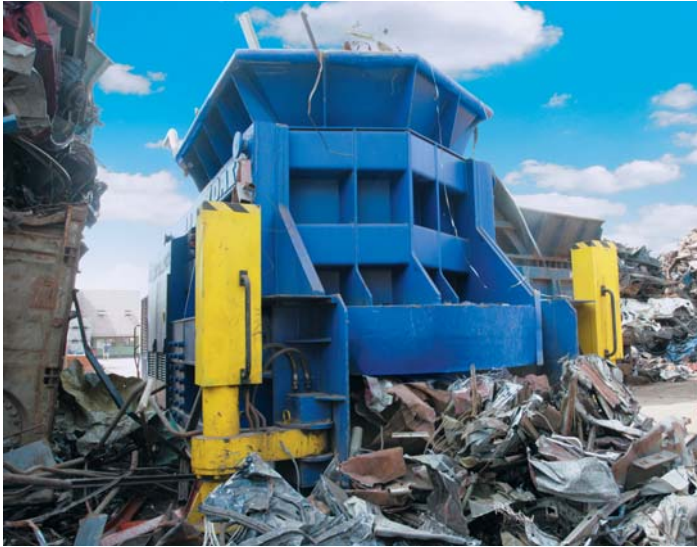
Output of processed scrap from the container shears
