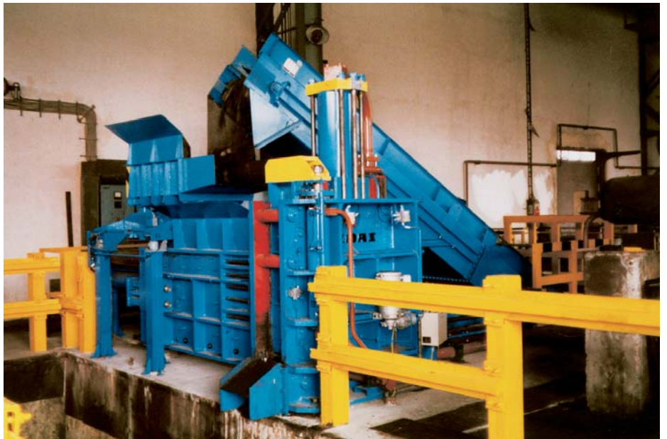
CPS 160 baling press at the pressing plant of a car body producer
