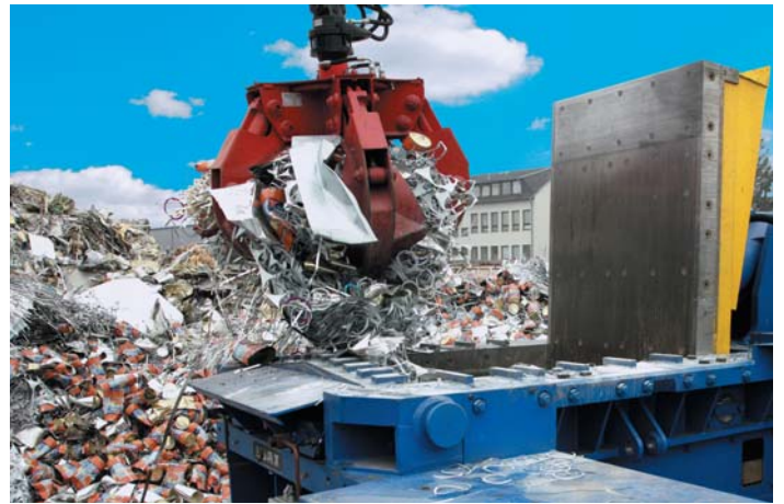
CPB 100 press efficiently processes municipal waste
