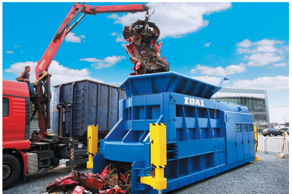
Loading scrap into the CNS 730 SM shears
