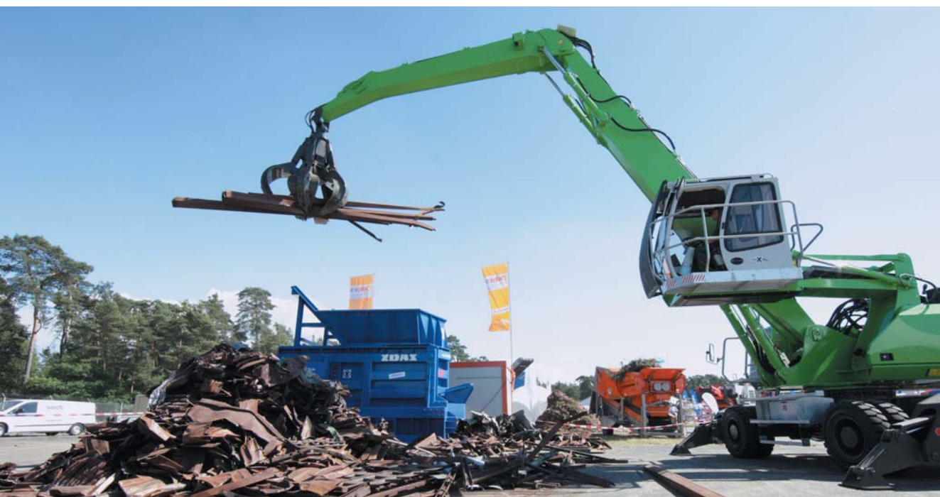
Loading the CNS 400 K shears with long scrap
