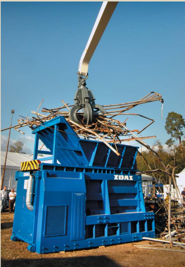
The CNS 400 K container shears with top hopper being filled with bar scrap
