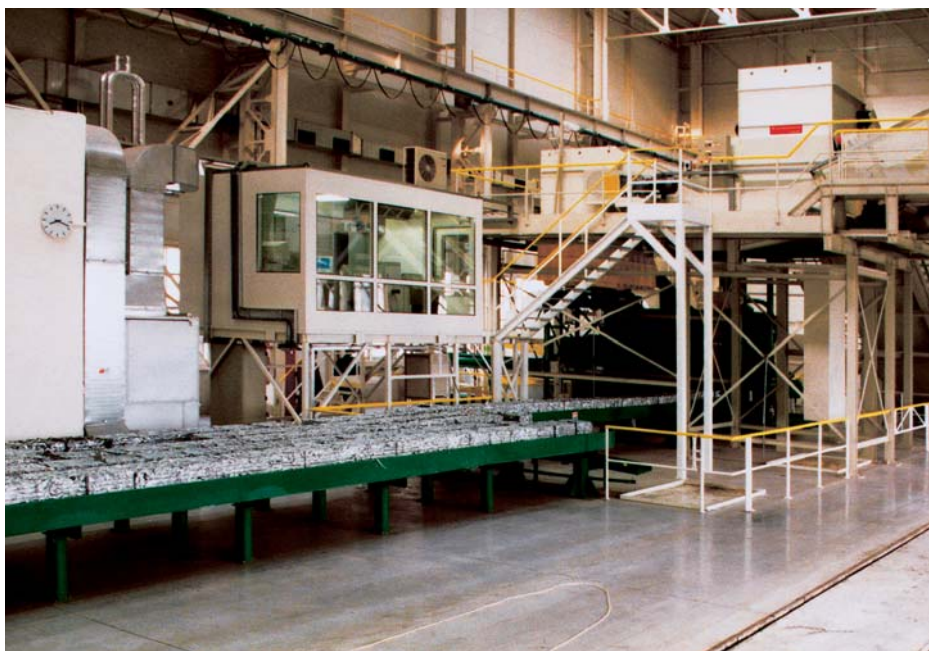
ZDAS CPS 320 baling press in a pressing shop of a large automotive manufacturer
