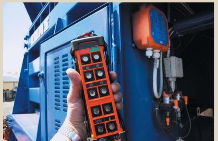
Remote control of the shears ensures safe operation and control by one operator
