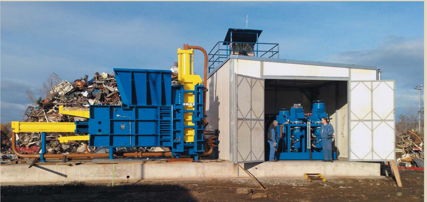
Press drive in a separate cabin
