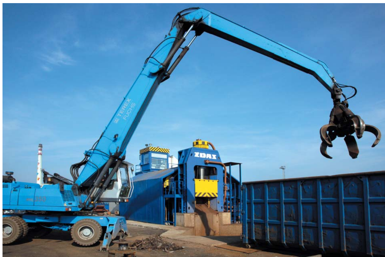
Workplace with CNS-PVM hydraulic shear
