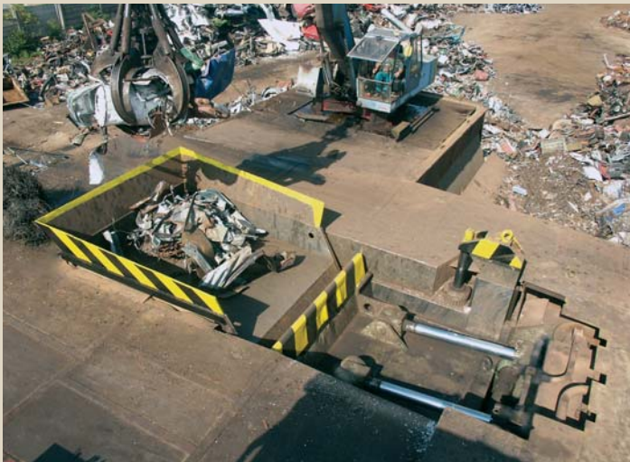
Opening the cover enables enough space for scrap feeding
