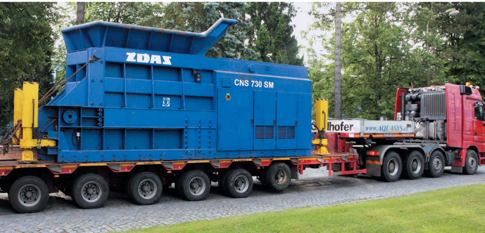
CNS 730 SM shears loaded on a flatbed trailer
