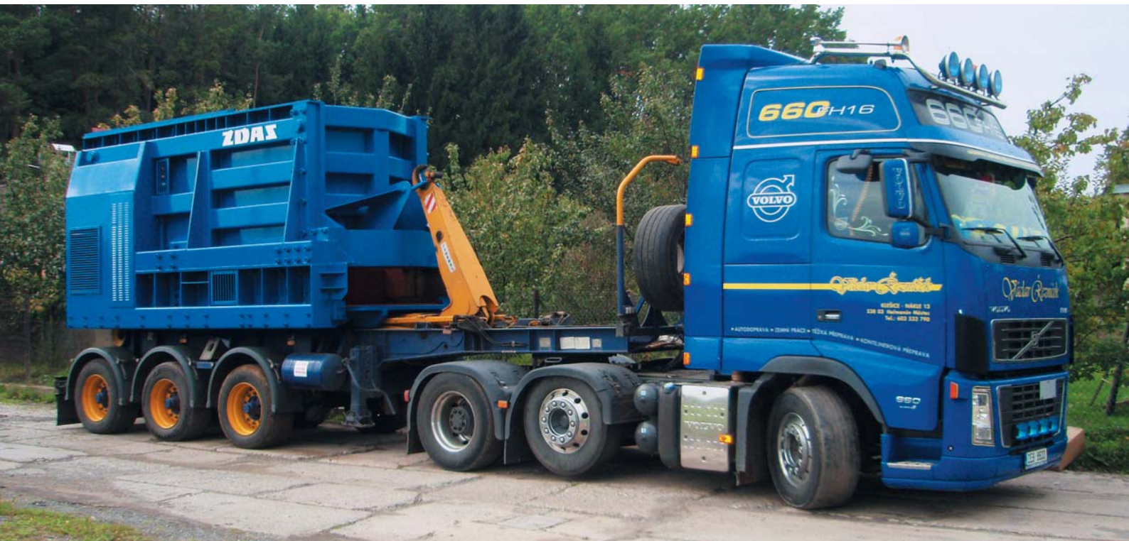
The CNS 400 K shears on a hooklift trailer
