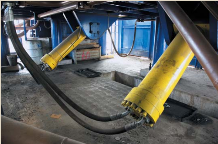
Hydraulic cylinders operating the folding cover
