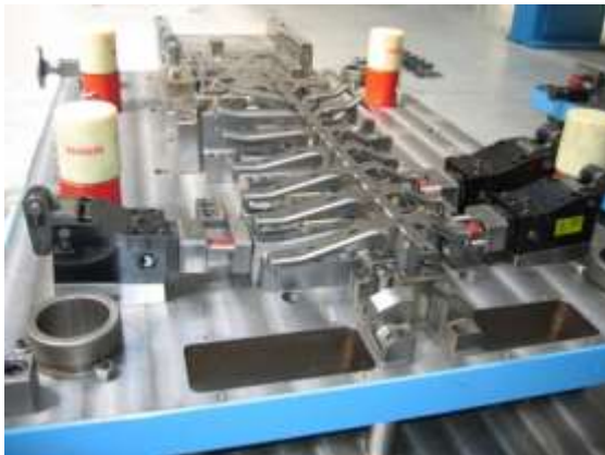
Progressive die 1560x1000x536 mm, 3000 kg
