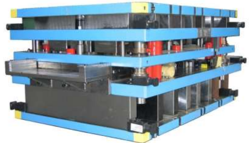
Progressive die 1600x1100x640 mm, 3000 kg
