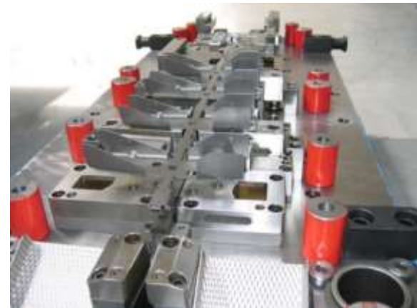
Progressive die 1210x520x550 mm, 1590 kg
