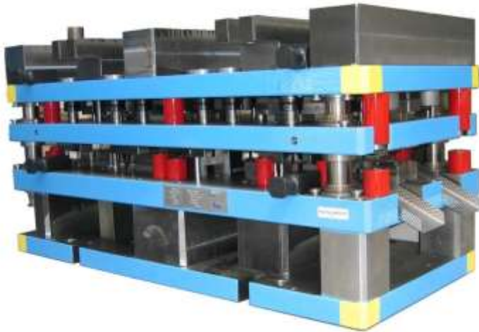
Progressive die 1210x520x550 mm, 1590 kg
