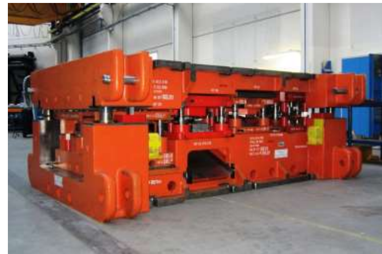
Transfer die Škoda SK482_Superb Combi 3235x2050x1150 mm, 15,4 t
